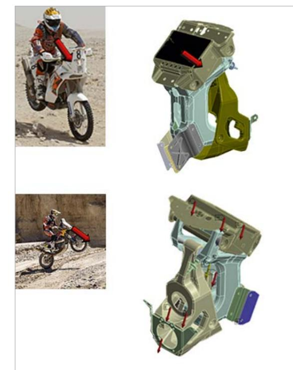
Fig. 2: Exemplary samples of load cases for component design - maximum load impact upper body on roadbook (top), operating load while jumping (bottom)
