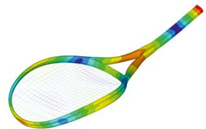
Second bending mode of a strung tennis racket
