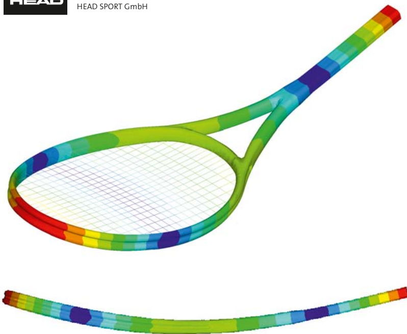
First bending mode of a strung tennis racket in elongation. Hitting the ball at the blue node line on the strings does not excite this mode. This is the sweet spot of the racket.
