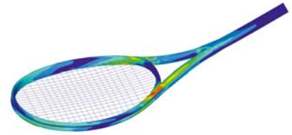
First bending mode of a strung tennis racket in tension.
