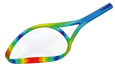
Torsion mode of a tennis racket illustrating how a non-center hit introduces torsion.
