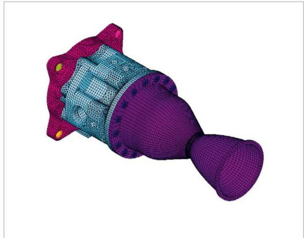
Fig.2: Thruster with combustion chamber
